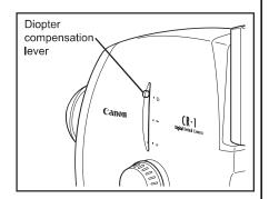
Note: When operating the diopter compensation lever, set it precisely to the 0, "—" or "+" position. If the lever is set to a position midway between two settings, fundus images will not be taken properly.
